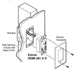
Figure 2-11 — Mounting the transmitter or receiver
